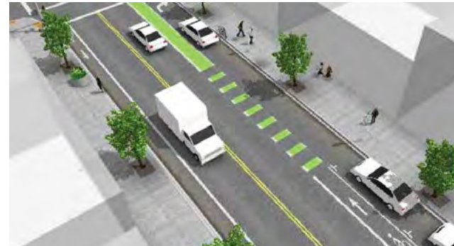
Enhanced bicycle facility treatments, such as colored bike lanes, improve visibility and safety for bicyclists
