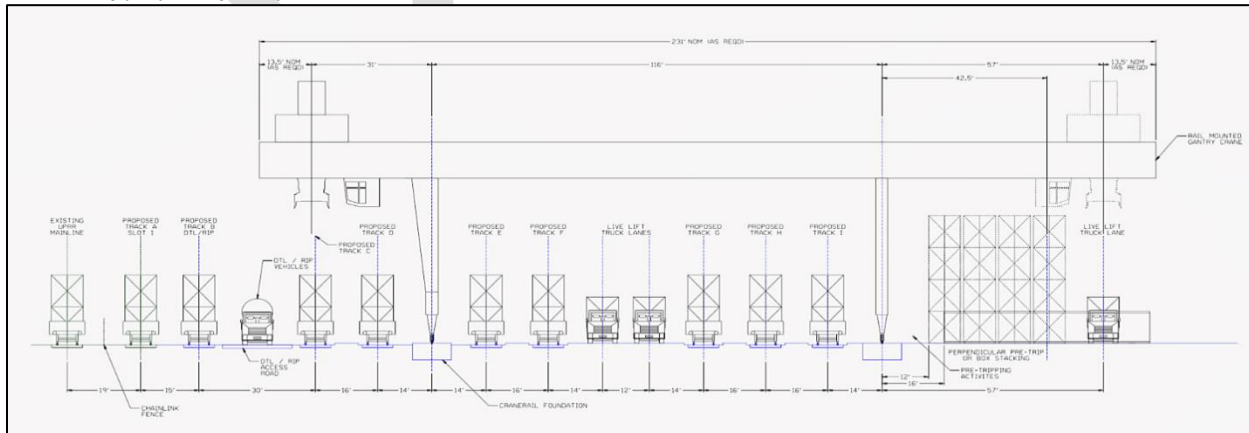
Section view of ramp and widespan crane
