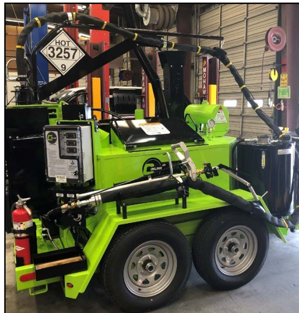
After Photo of New Crack Seal Machine
