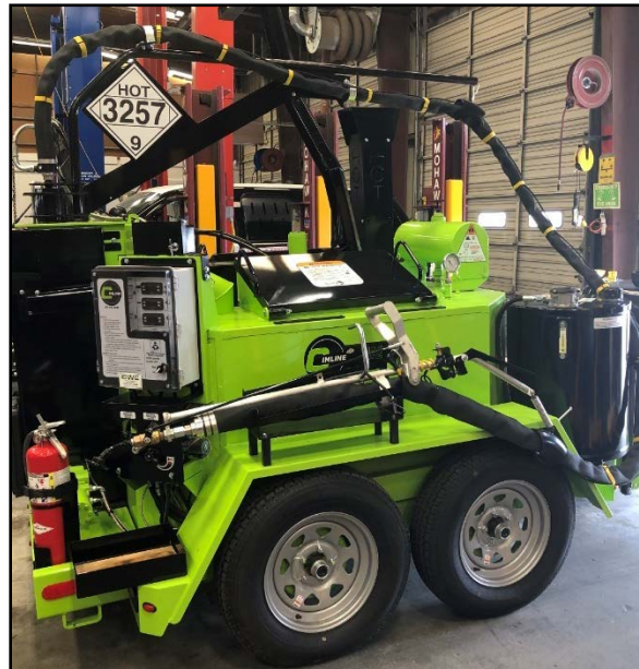
After Photo of New Crack Seal Machine
